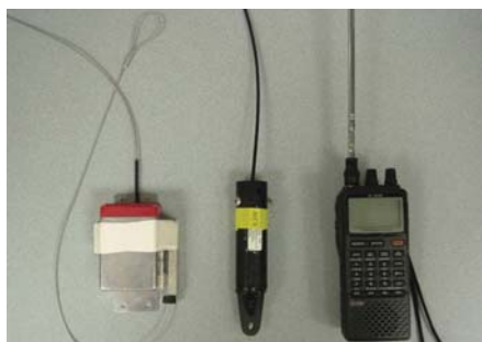
Remote trap monitors alert field specialists, wildlife managers, and others when animals are captured in traps.
